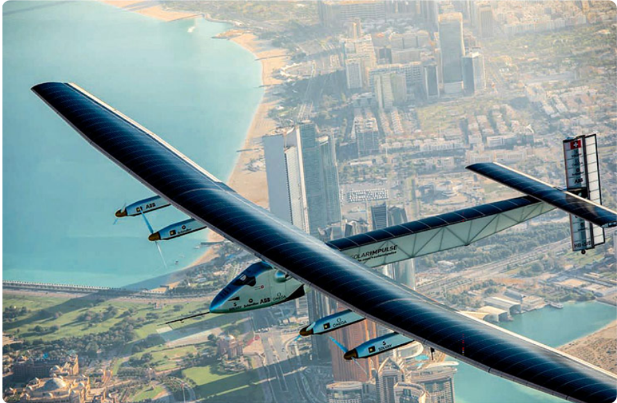
A nice view of the solar panels is visible here as Solar Impulse 2 undertakes preparation flights over Abu Dhabi (UAE).
