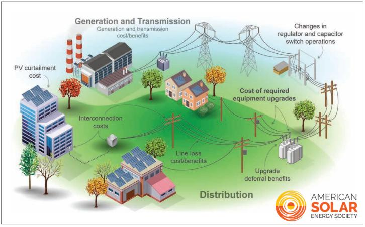
NREL's analysis of hosting capacity upgrade costs is one component of the overall cost-benefit equation for distributed energy resources that also includes the installed cost of the distributed photovoltaic (DPV) system, transmission and bulk system costs and benefits, and a variety of other potential values.
