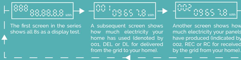
Some meters will have another screen that indicates power currently being sent to the grid (i.e. generated by your panels) with the unit W or kW (instead of kWh). Others may use arrows or sliding dashes to denote the direction of electricity flow, where to the right means consumption and to the left means generation. If there is a screen showing your current production and it is non-zero, then your system is working.
